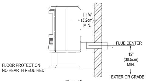
Figure 37 Minimum Exterior Grade Dimension - Unit With Pedestal
